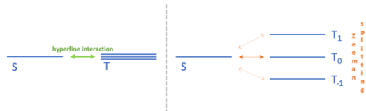
Figure 4. Zeeman splitting. Picture adapted from Kuno et al. (2015) [42]
